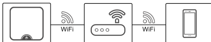
Figure 7-2 Mobile phone connecting to the SUN2000L over a router
